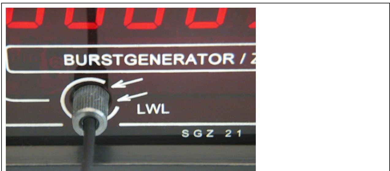
Figure 6: Optical fibre connection on the SGZ 21.
