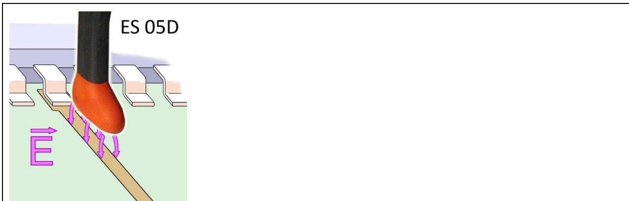
Figure 35: The electric field of the field source couples to the conductor loop and feeds a current pulse into this loop).
